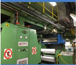
We use high speed stack and CI Flexo presses capable of printing 4 color line work or up to 6 color process designs.
